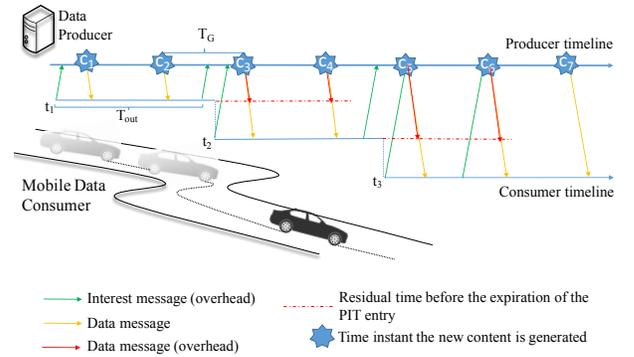
Fig. 4. Message sequence chart showing *Interest* and *Data* packets exchanged when the *push-based* approach is used.
