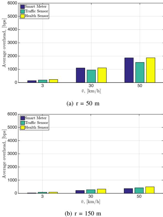
Fig. 5. Communication overheads related to the pull-based approach, when the average coverage area of network attachment points is equal to (a) 50 m and (b) 150 m.
