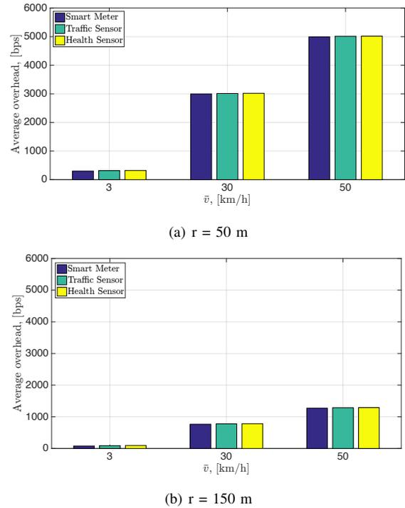
Fig. 6. Communication overheads related to the push-based approach, when the average coverage area of network attachment points is equal to (a) 50 m and (b) 150 m.
