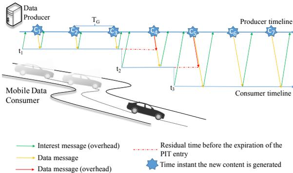
Fig. 3. Message sequence chart showing *Interest* and *Data* packets exchanged when the *pull-based* approach is used.
