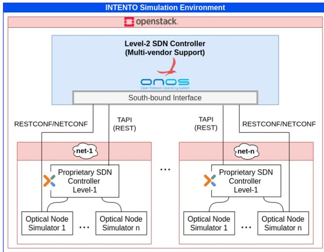
Fig. 2. The developed simulation framework.
