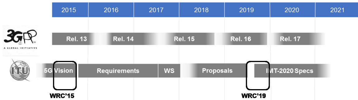
Figure 15-1. ITU-R process and its alignment with 3GPP specifications.
