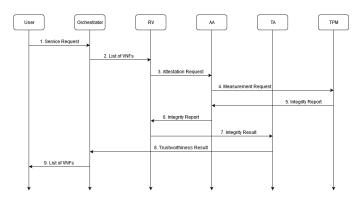
Fig. 4. Sequence Diagram of the Attestation procedure of the service chain
