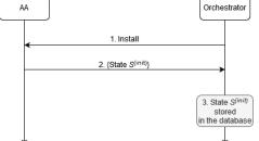
Fig. 2. Sequence Diagram of the VNF Installation procedure
