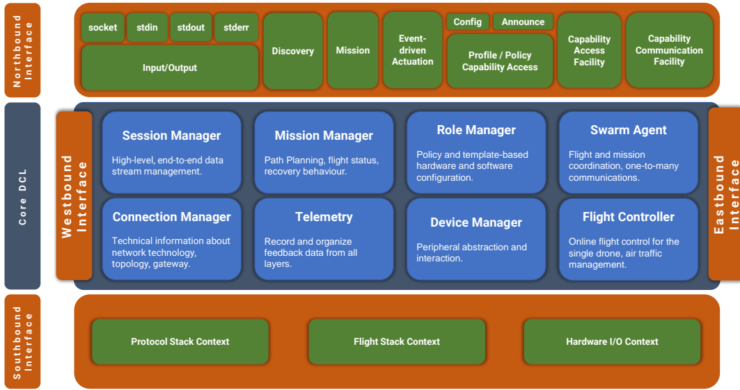
Fig. 5: High level architecture of the DCL.
