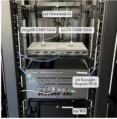
Fig. 2. Hardware setup for the experimental evaluation of integrated T/NTNs.
